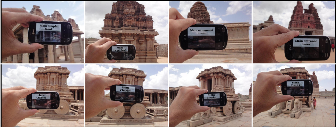
Figure 8. An application of the compact search index structure for tourism. Mobile phone localizes and gives details of what it sees without the help of external network. The first row shows usage at different locations and monuments; the second row demonstrates the robustness of the approach to view-changes of a particular monumental structure.
