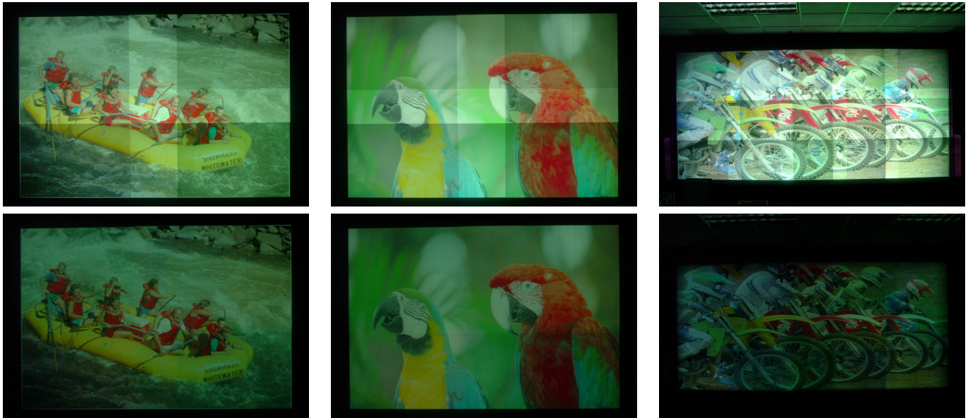
Fig. 13. The top row shows the image before correction and the bottom row shows the image after luminance matching. Left and middle: Digital photograph of a 2 \times 2 array of projectors. Right: Digital photograph of a 5 \times 3 array of projectors. In this case, the image after correction was taken at a higher exposure.
