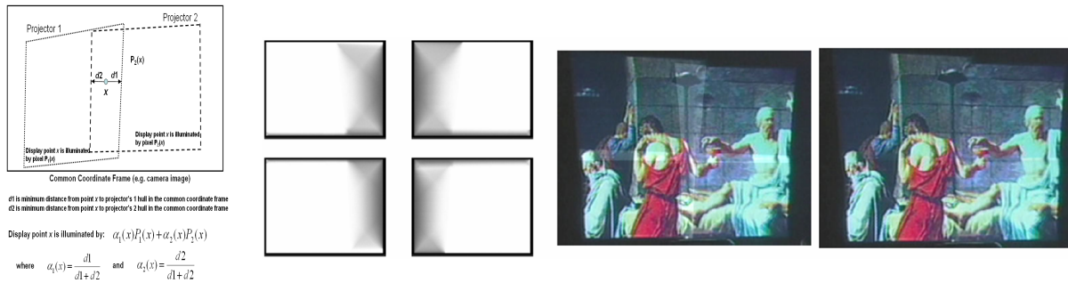
Fig. 8. Blending Techniques: (Left) The intensity at any pixel x in the overlapped region of two projectors, P_1 and P_2 , is the combination of the intensity of P_1 and P_2 at x . (Right) The resulting alphamasks computed for four projectors.
