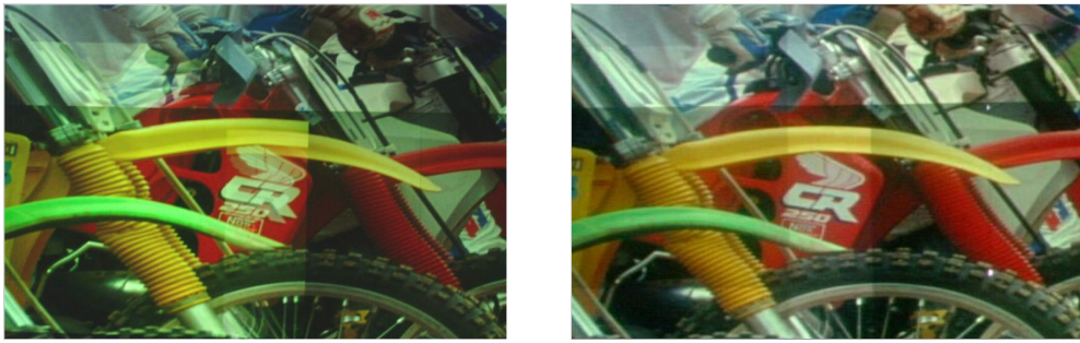
Fig. 2. Left: This image illustrates the geometric misalignment problem at the boundary of two overlapping projectors. The geometry is noticeable unaligned. Right: This image shows the final seamless imagery of the same projector alignment. Such registration that is the goal of geometric registration methods.
