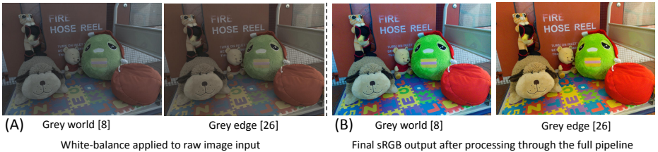
Fig. 6. (A) White-balancing algorithms applied on raw images. (B) sRGB output of white-balanced images.
