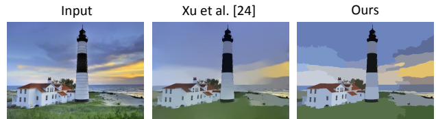
Figure 11. This figure shows the drawback of strong L_0 gradient minimization for images. For the task of image smoothing, the method by Xu et al. [24] may be more appropriate, as our method will introduce more noticeable color quantization into the result.
