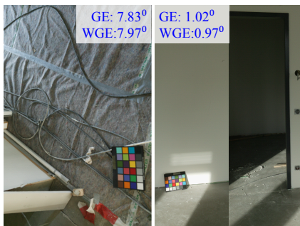
Fig. 5. These images (from [40]) of different scenes are taken in the same illumination, but the error in illumination estimation using spatial domain methods is quite different for the two images. The labels in the top corners of the images show the angular errors of the grey edge (GE) and weighted grey edge (WGE) algorithm.
